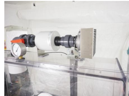
HEPA exhaust filter
